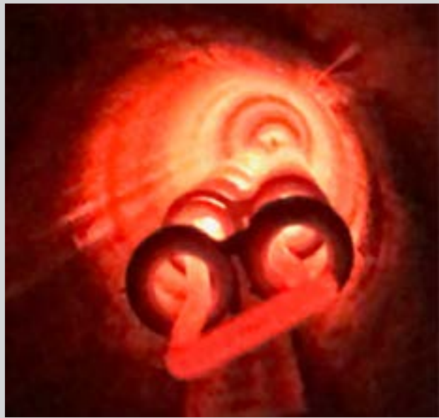
Our FlexHeater ® thermal conduction heating service element glows in a pipe.
